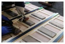
b) Removing by a scraper
