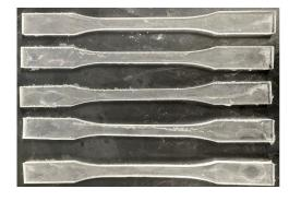
Fig. 3 Cured epoxy resin tensile specimen
