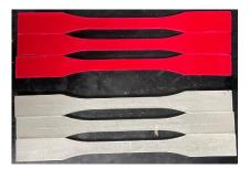
(a) Tensile samples with phosphors
