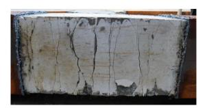
(a) Tensile side of sandwich concrete
