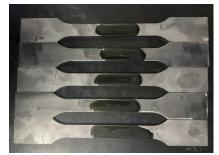
(b) Steel samples coated with the GQDs-epoxy resin composites
