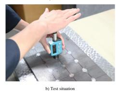
Fig. 11 Leeb hardness test device and test situation
