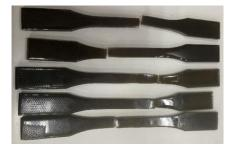
Fig. 11 Tensile samples after fracture
