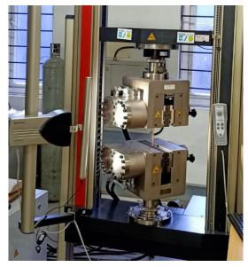
Fig. 5 Electromechanical testing machine (Zwick/Roell Z100 kN)
