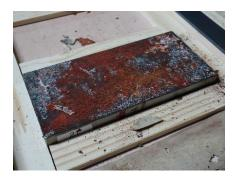
Fig. 5 Specimen after IH paint-coating removal
