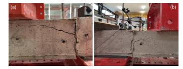
Fig. 5 Cracks on the middle slab – vertical surface of the test specimens: (a) R1 series, (b) R2 series
