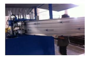
(a) Roofing plate bending and arc processing
