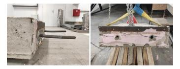
Fig. 6 Construction joint upon the testing
