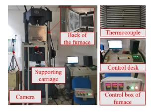
Fig. 6 Test setup
