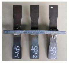
(b) Welded joint plate specimen
