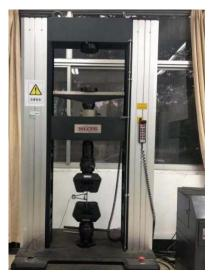
Fig. 1 UTM5305 electronic universal testing machine
