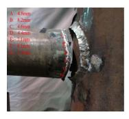
(a) Brace and weld penetration breakpoints
