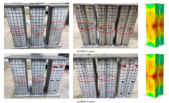
Fig. 8 Comparison of failure modes of axial compression short columns
