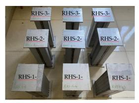
Fig. 2 Axial compression short columns
