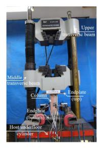
Test machine QD1 Endplate (Upper) S6 S5 1 1/4 Built-up column 1-1 2-2 2 2 3 3 1/4 Endplate (Bottom) Arrangement of LVDT 3-3 Arrangement of strain gauges
