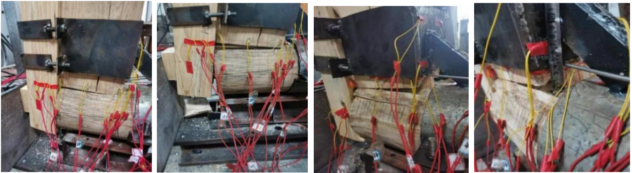
(a) Initial loading stage (b) Onset of fiber tearing at the mortise (c) Progressive tenon pull-out under cyclic loading (d) Localized crushing & separation at joint interface
