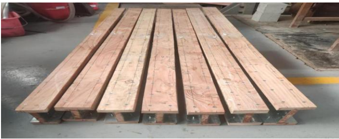
Fig. 2 Finished steel-wood combination beam member
