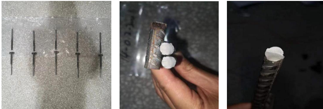
(b) Fatigue failure of specimens
