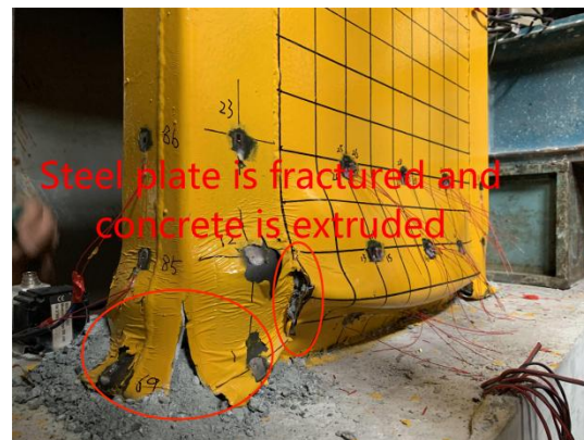
(b) Failure mode of steel plate in SCW-2
