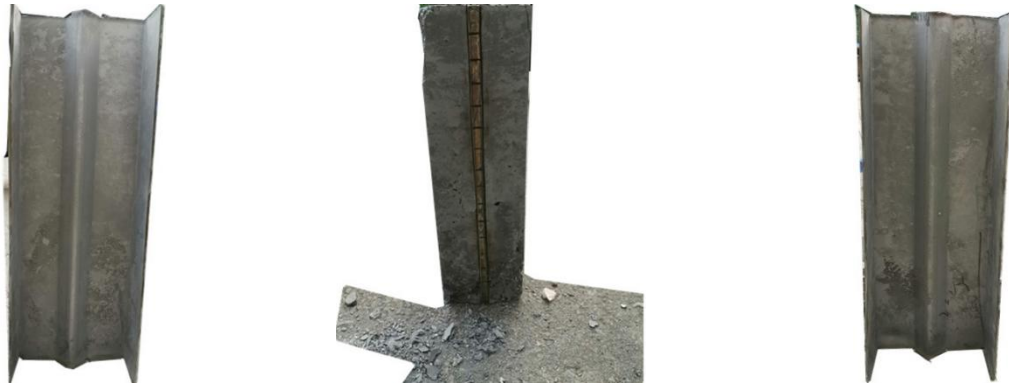
Fig. 6 The failure characteristics of RB component
