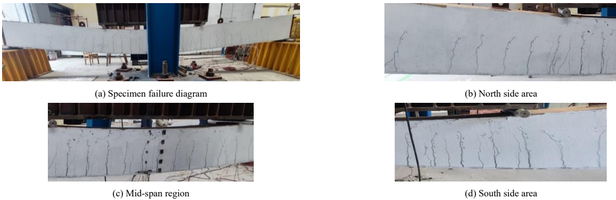
Fig. 5 Final failure state of specimen PECB2
