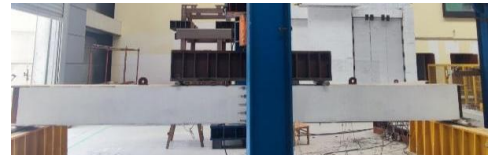
(b) Loading device of PECB2 and PECB4 specimens
