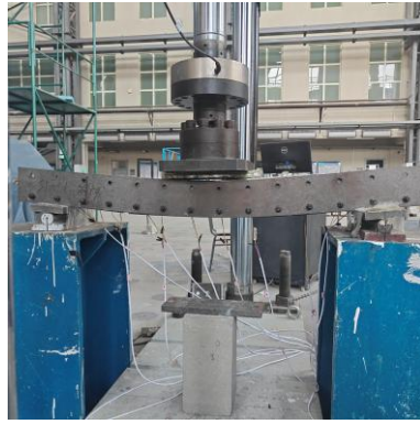
Fig. 21 The global buckling
