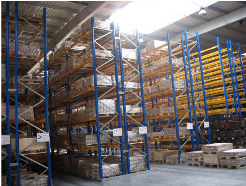
Figure 1. Typical Pallet Racks Configuration
