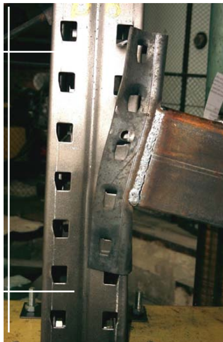
Figure 12. Deformation of Panel Zone
