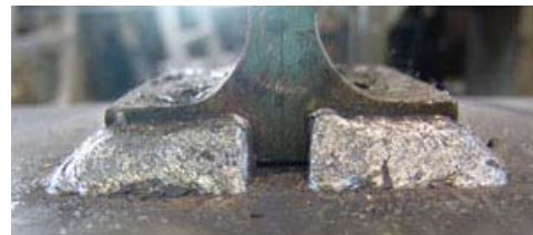
(c) deformed column and detail of fillet weld (specimen C1)
