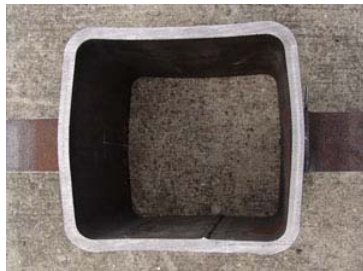
(c) deformed column and detail of fillet weld (specimen C1)
