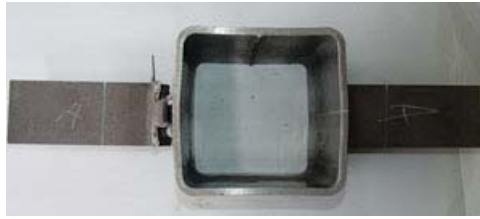
(a) rupture of bracket flange and fillet weld (specimen A3)
