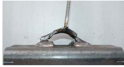
(a) rupture of bracket flange and fillet weld (specimen A3)
