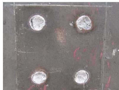
(d) deformed column and fracture surface of plug weld (specimen D3)
