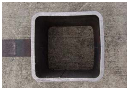
(d) deformed column and fracture surface of plug weld (specimen D3)
