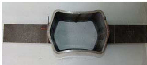
(b) deformed column and flexure of tee bracket flange (specimen B2)
