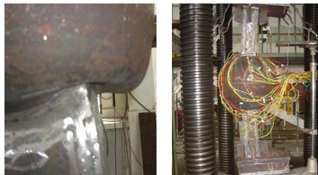
Figure 10. Deformed Shape of Specimen 1
