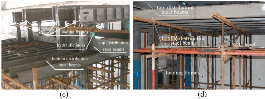
Figure 4. Loading Mechanism and Test Set-Up
