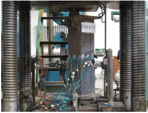
Figure 3. The Typical CFST Column Specimen before Testing
