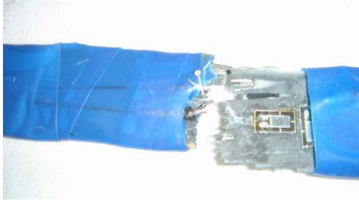
Figure 3. Typical Failed CFRP Coupon
