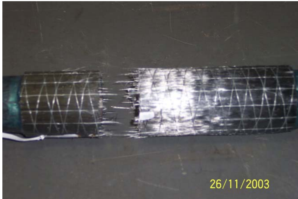
Figure 4. Failure Mode of the Test Specimen[1]
