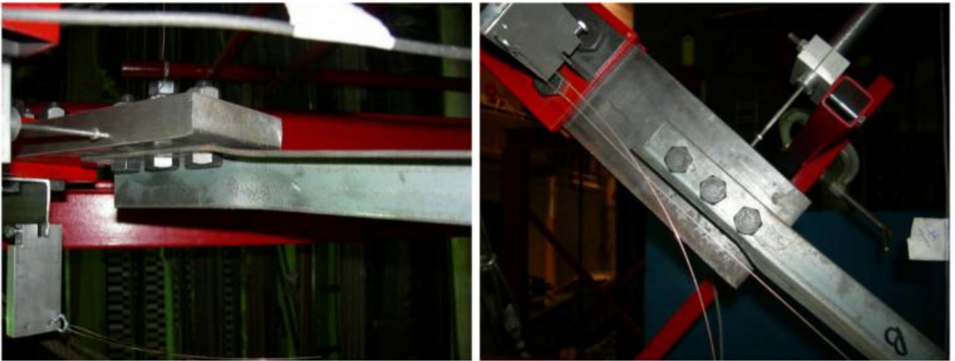
Fig. 12 Local failure of test specimens (2 and 3) [24]
