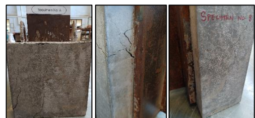
Fig. 15 Crushing of concrete in specimen 8 (CPS-2 nd )
