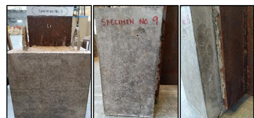
Fig. 16 Crushing of concrete in specimen 9 (CPS-3 rd )
