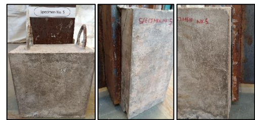
Fig. 14 Crushing of concrete in specimen 5 (CPS-1 st )
