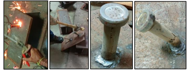
Fig. 5 Welding and bend test of shear connector
