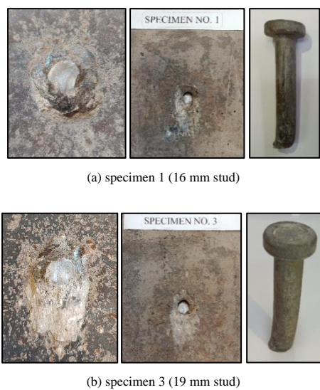
Fig. 12 Failure of headed stud shear connector
