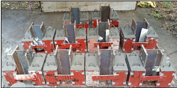
Fig. 7 Ten number of specimens after concreting
