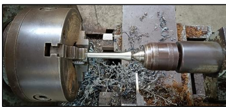
Fig. 4 Preparation of CPS-shaped stud using Lathe machine
