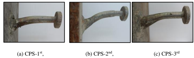
Fig. 13 Deflected shape of CPS-shaped stud
