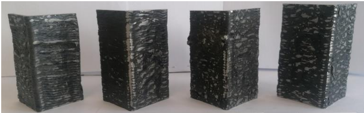
Fig. 3 The stub column samples after being removed from the substrates and with balling roughly removed (from left to right, samples EL1, EL2, EH1 and EH2)
