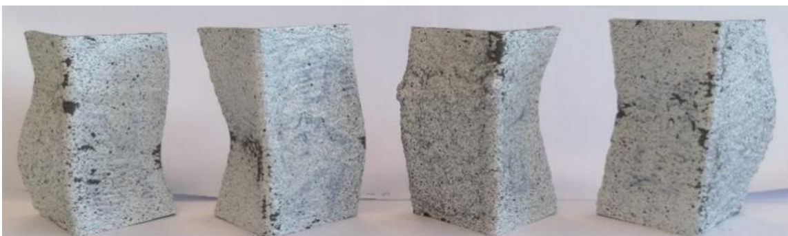
Fig. 10 The buckled stub columns after testing (from left to right, samples EL1, EL2, EH1 and EH2)
