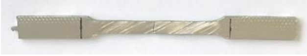
Fig. 4 The sample TH-45-2 after testing. It has been placed back together and there are surface deformations visible at 45° to the length of the coupon, corresponding to the fact that the coupon was extracted from the WAAM build at 45°.
