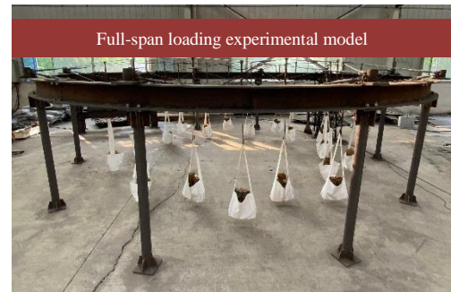
(a) Full-span loading experiment
