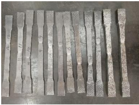
Fig. 4 Coupon test of specimens
