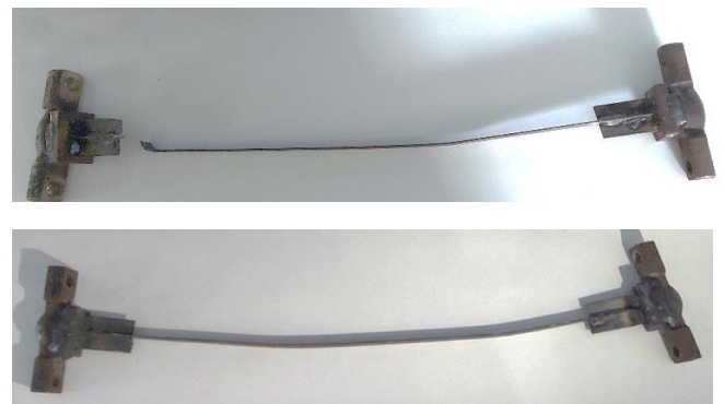
Fig. 8 Failure pattern of core part for specimen 1 (above) and specimen 2 (below)
