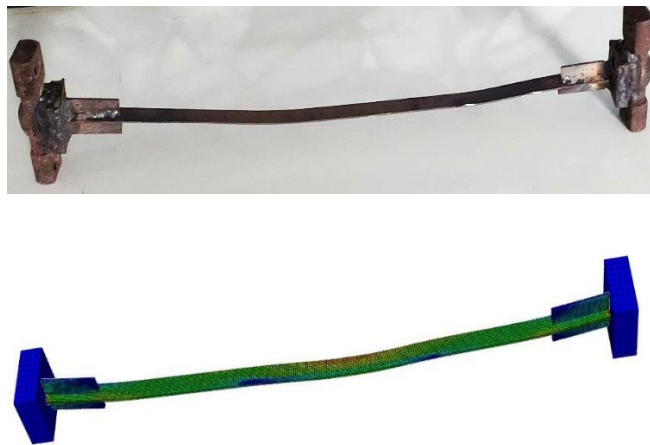
Fig. 17 Failure pattern observed in specimen 2 (experimental and FE)
