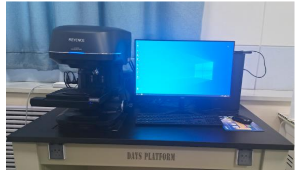
Fig. 8 The Keyence VK-X1000 3D noncontact morphology scanner
