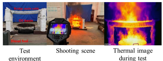
Fig. 20 Realistic fire test scenario of bridge cables
