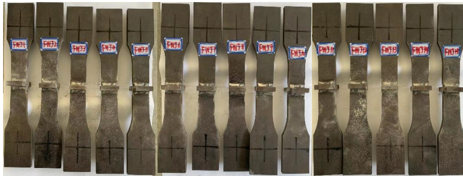
Fig. 2 Specimens of Q460C steel fillet weld cruciform joints
