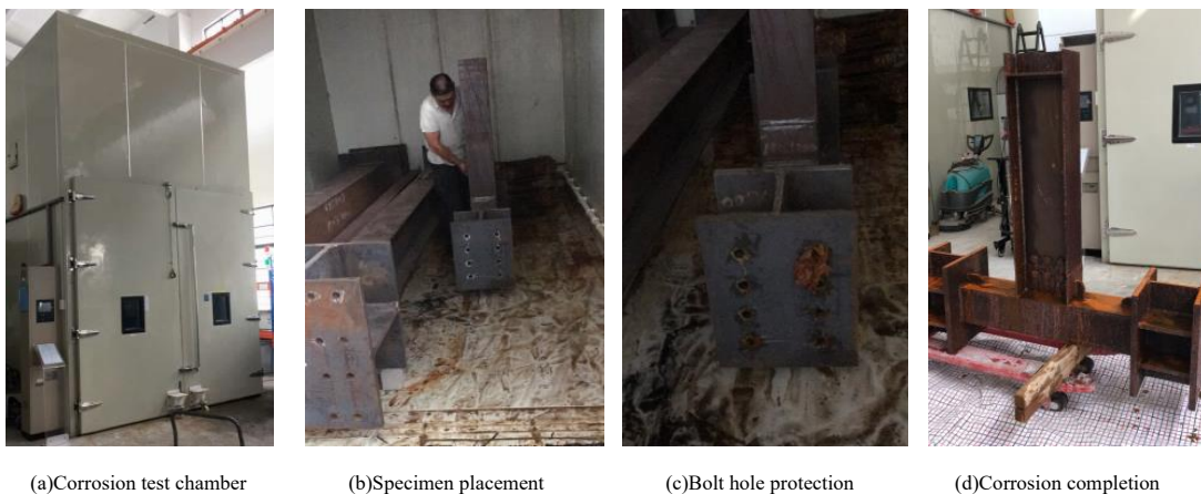
Fig. 4 Corrosion process of the specimen LZ-2
