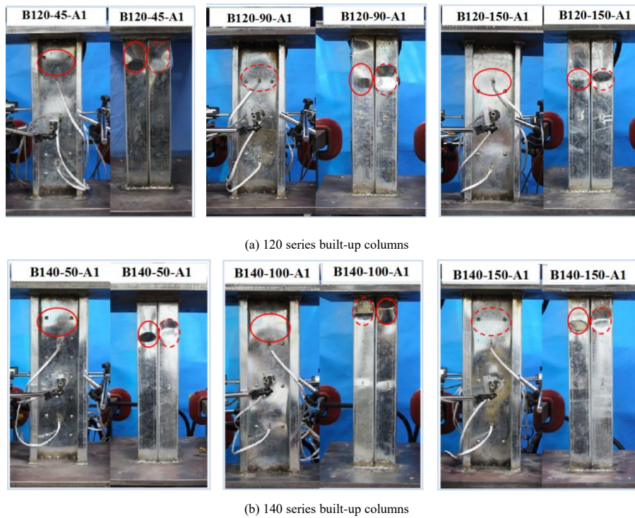
Fig. 11 Buckling characteristics of test specimens
