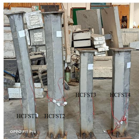
Fig. 12 Distorted shape of HCFST slender columns
