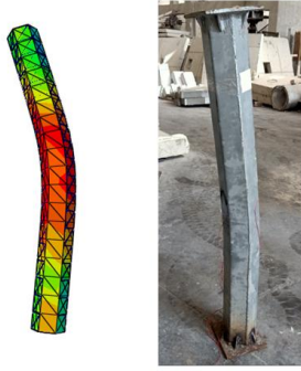
Fig. 17 Mode of failure FE and test results for the HCFST1 slender column specimen
