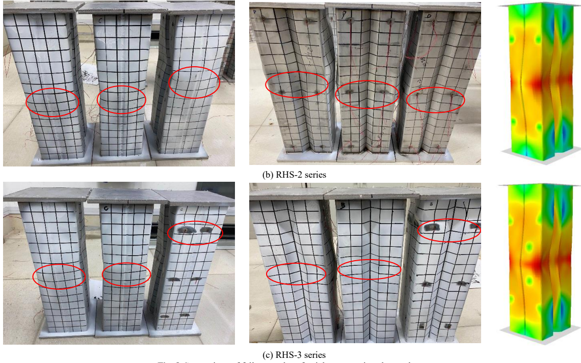
Fig. 8 Comparison of failure modes of axial compression short columns
