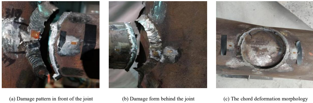
Fig. 6 Failure mode of joint specimen GX-2
