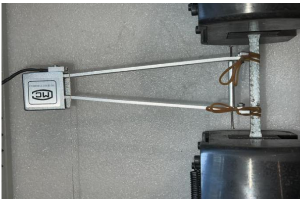
Fig. 11 Using an extensometer to measure tensile deformation
