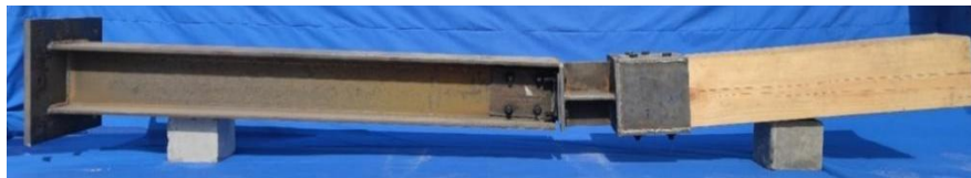
(a) Deformation pattern of specimen M-SWMC-J-2 test
