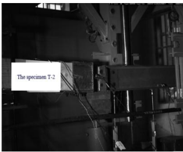
(a) The head is not in contact with the specimen
