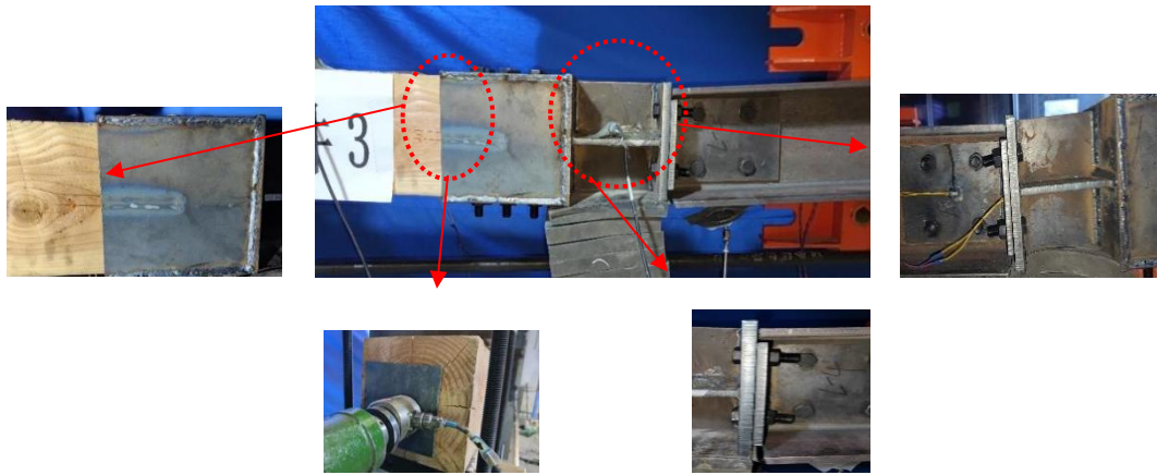
Fig. 16 Deformation mode of specimen M-SWMC-S-3 after impact
