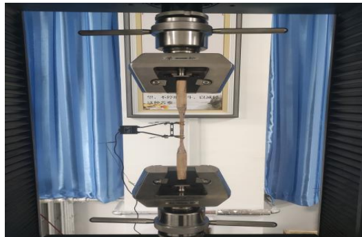
Fig. 3 Tensile strength test of wood along the grain
