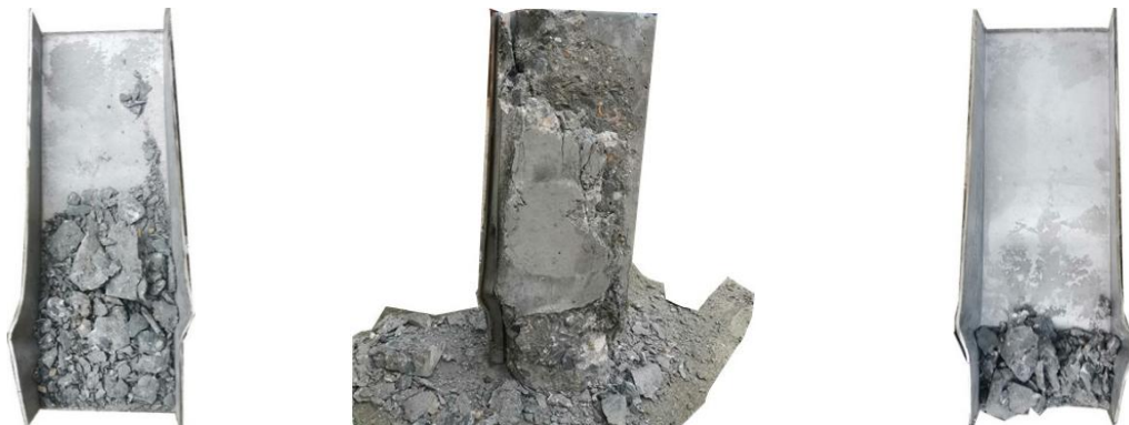
Fig. 5 The failure characteristics of RA component
