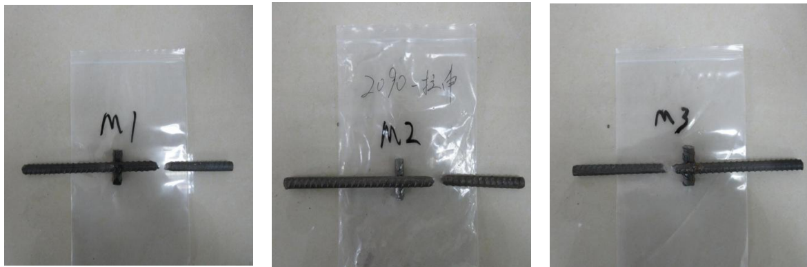
(a) Static failure of specimens
