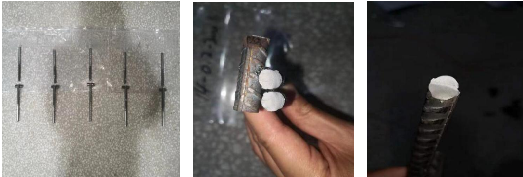
(b) Fatigue failure of specimens
