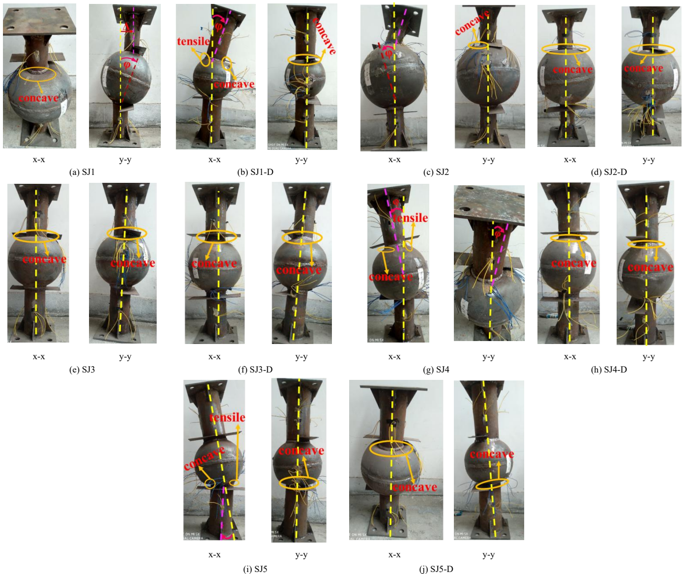
Fig. 16 Actual view of specimen destruction
