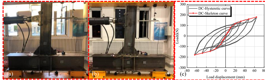
Fig. 3 Test phenomena for \Delta = (a) 16 and (b) 64 mm. (c) Hysteresis and skeleton curves
