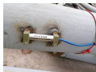
Fig. 7 The strain sensor
