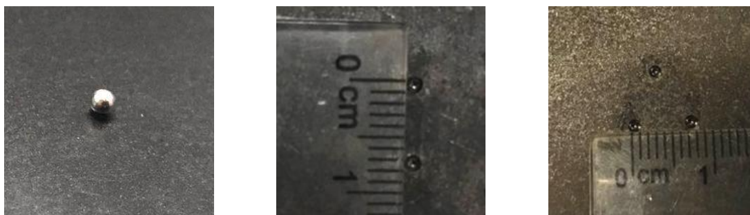
Fig. 4 Test effect diagram of embedding into 1.5mm particles
