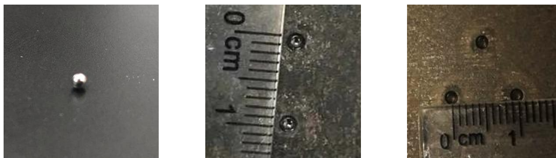
Fig. 6 Test effect diagram of embedding into 2mm particles
