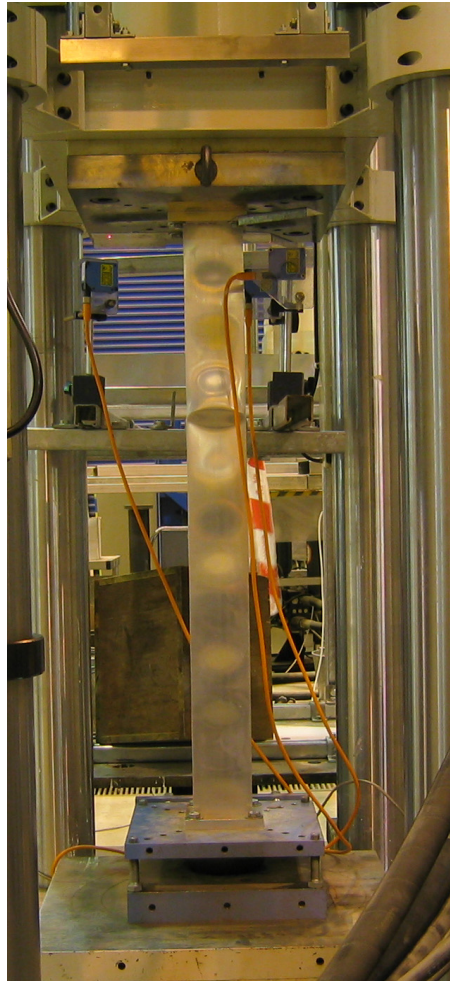
Figure 2. Column Specimen Failed by Local Buckling
