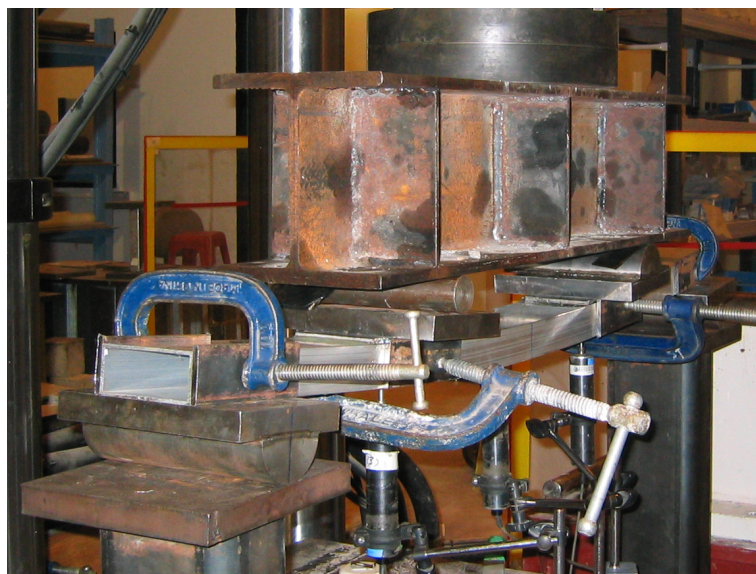
Figure 4. Flexural Buckling of Beam Specimen R2-PB
