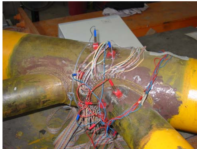
Figure 5. ACPD Test Set-up and Location of the Crack
